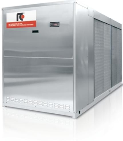
Outdoor unit for the production of chilled water with hermetic rotary Scroll compressors, axialflow fans, shell and tubes exchanger and thermostatic expansion valve. External panels in Peraluman and structure in aluminium sections. The range is equipped with two compressors on two independent refrigerant circuits.
